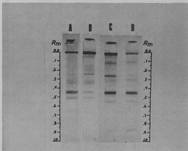
Figure 2. Disc electrophoretic pattern for actomyosin. A = 0.05 ml of beef actomyosin preparation containing 6.0 mg protein/ml. B = 0.05 ml of low ionic strength-treated actomyosin containing 6.0 mg protein/ml. C = 0.10 ml of DTT reduced sample from B (above) containing 5.5 mg protein/ml. D = 0.05 ml of DTT reduced actomyosin preparation containing 3.0 mg protein/ml
